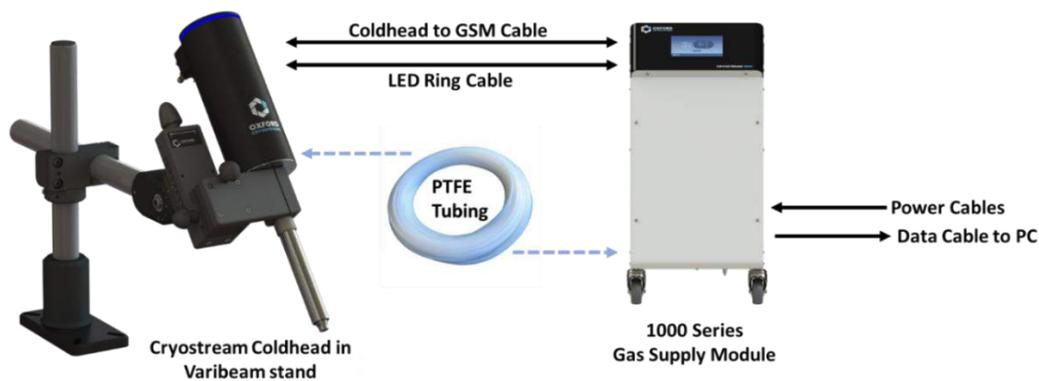
Figure 6.1 Simplified schematic of the Cryostream set up
