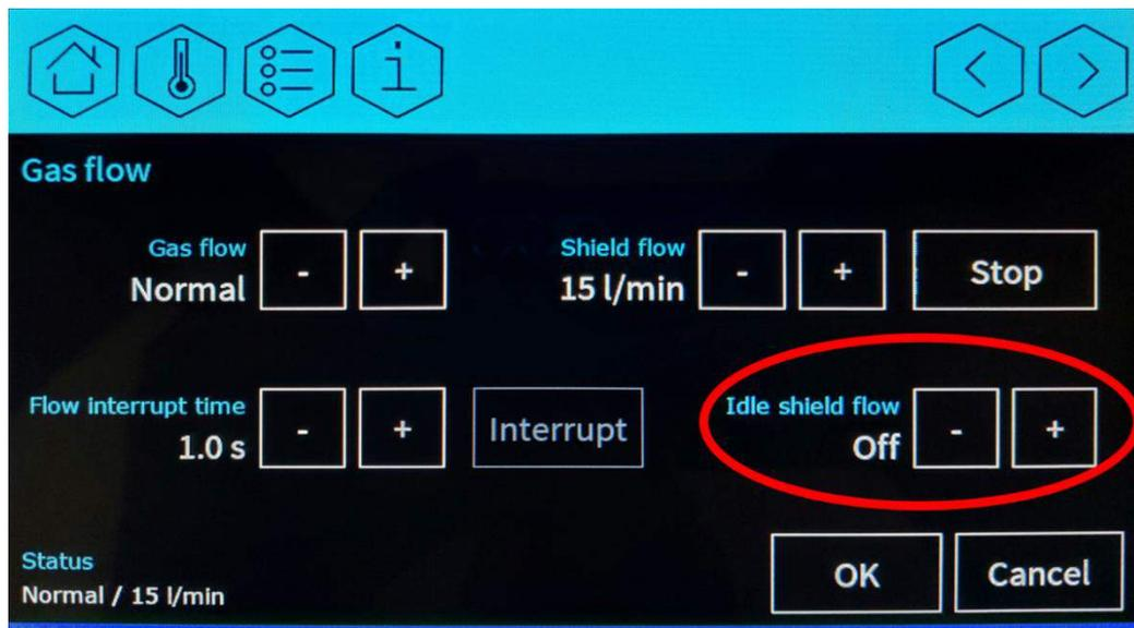
**Figure 7.8 Idle Shield flow settings on the controller**
