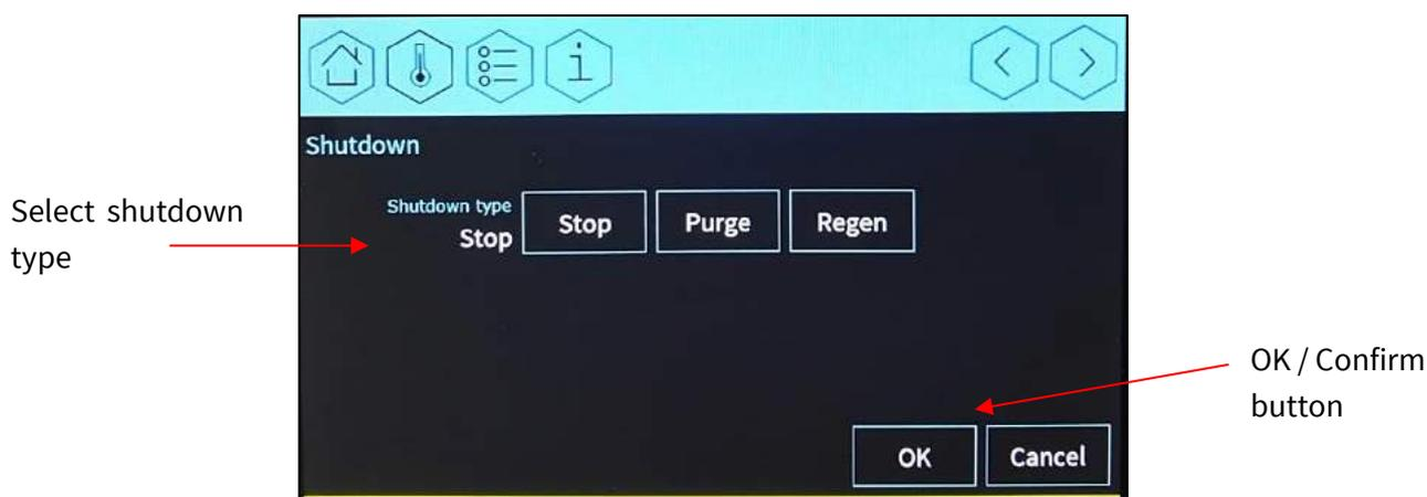
Figure 7.13 Command screen 3 showing shut-down options
