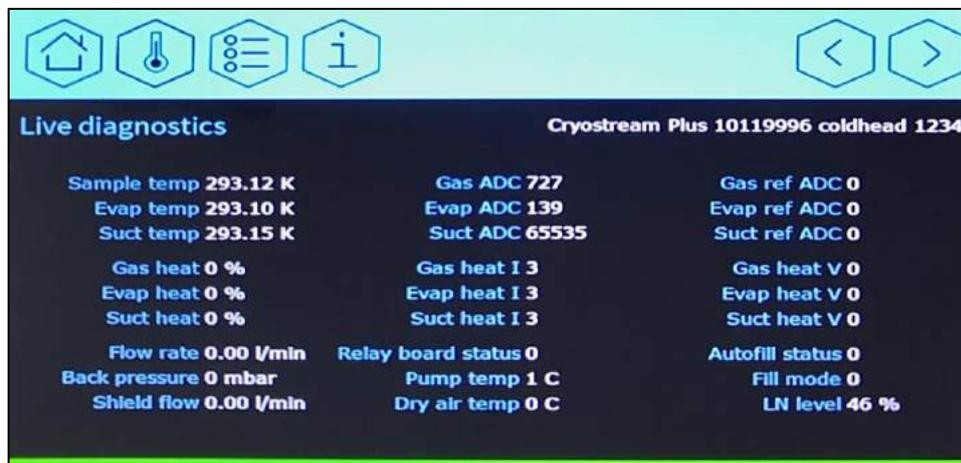
Figure 7.14 Info screen I: Sensors and heaters
