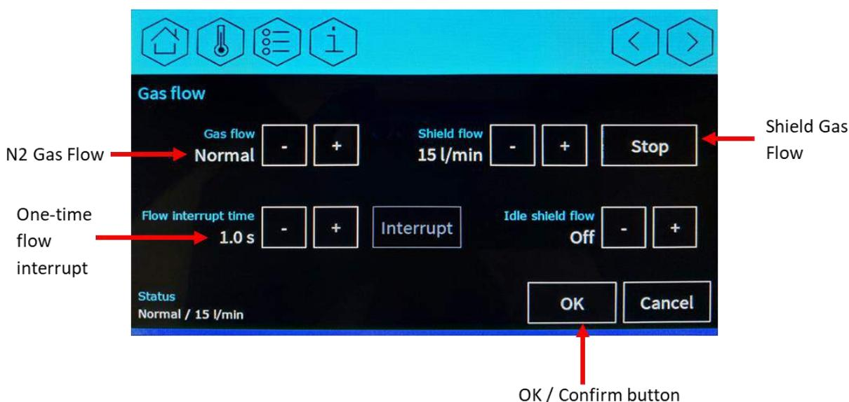
Figure 7.12 Command screen 2 showing gas flow settings
