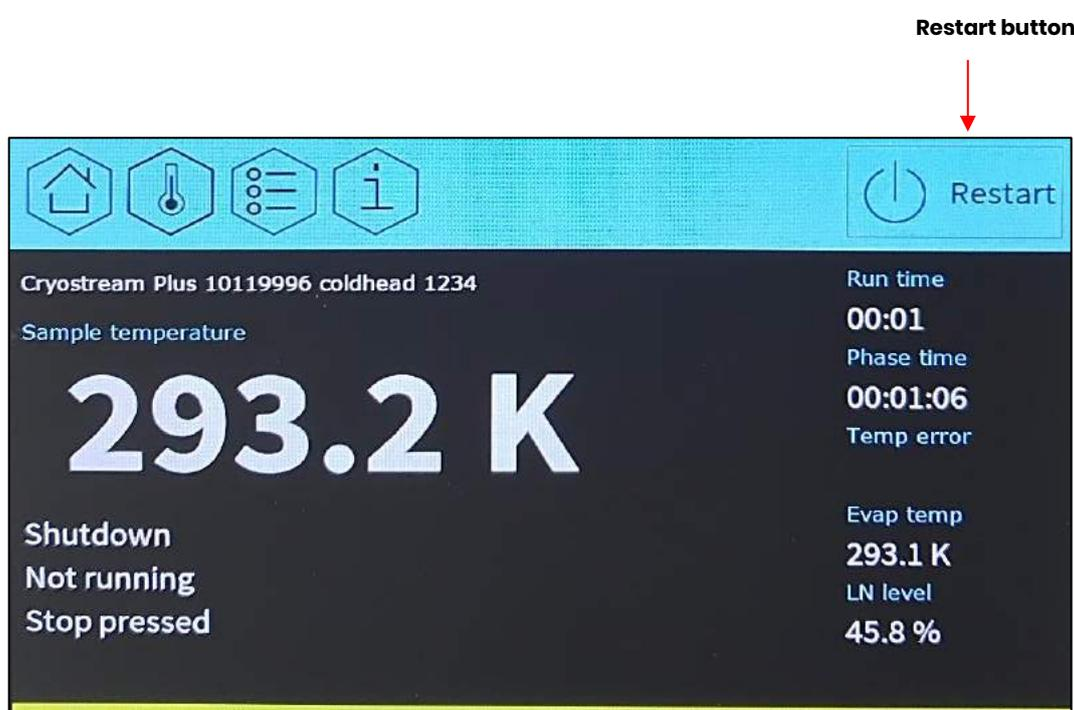
Figure 7.10 Home screen when Cryostream is stopped
