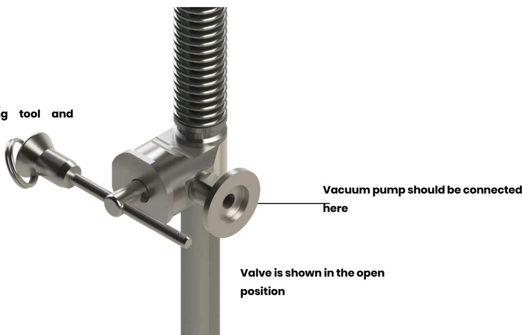
Figure A7 Pump out port
